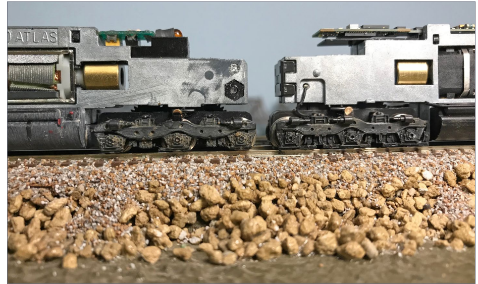
12. Side-by-side truck comparison. Factory SD35 truck is on the right, and the modified SD20 truck on the left (minus the middle brake cylinder and brake shoes).
