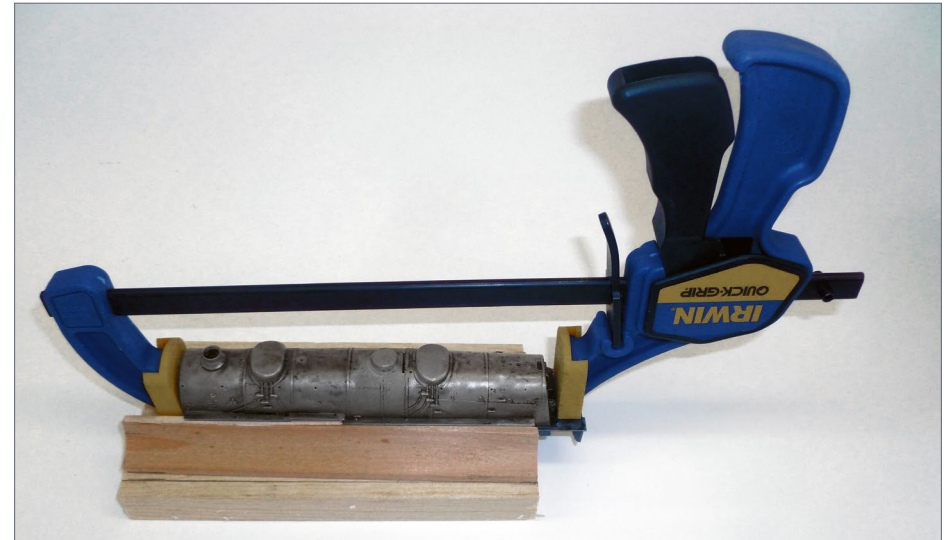
12. I built a jig to glue the two pieces back together. A clamp holds them in place.
