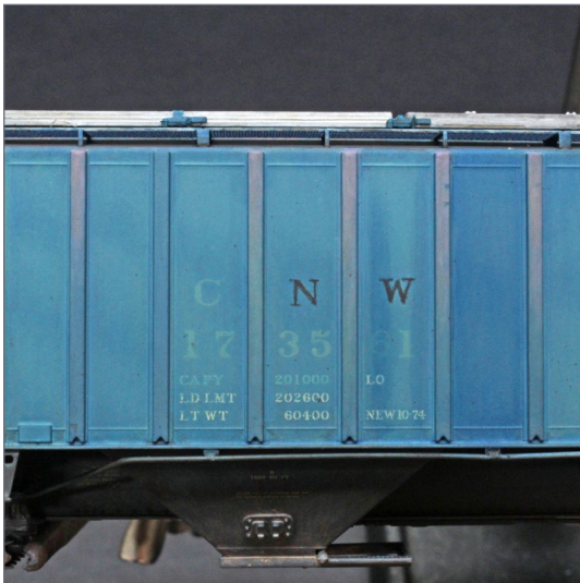
52. A steady hand is required to trace over the reporting marks with black paint.
