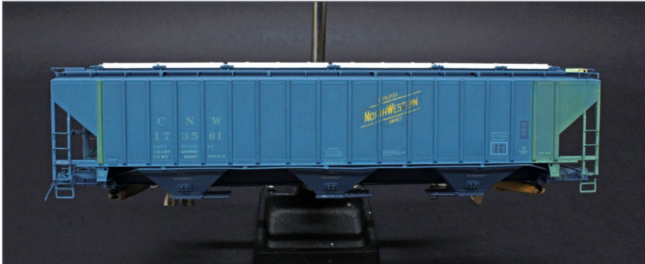
25. After four washes the green areas are opaque enough.
