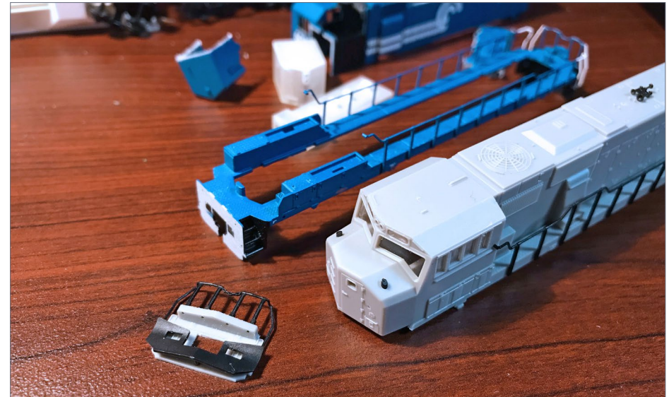
9. Front pilot reclaimed from an Atlas SD60M shell solved the railing, anti-climber, and plow part of the puzzle all at once.
