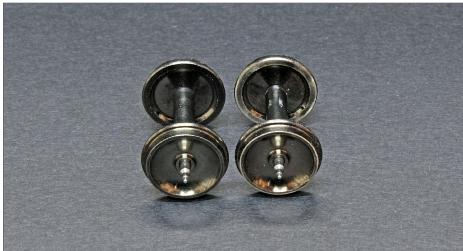
6. Compare the sanded wheels on the right to those that haven't been treated.
