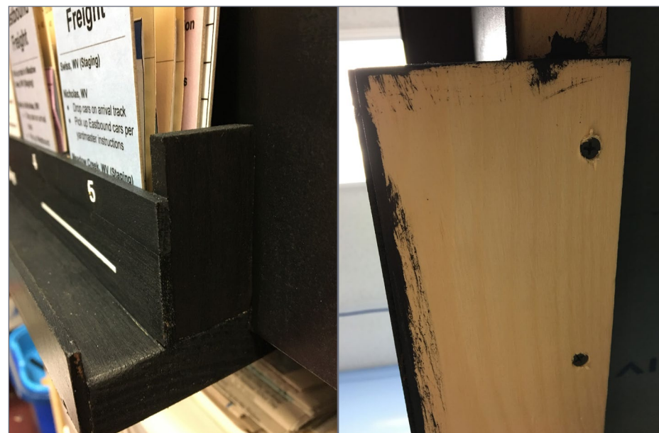
3a,b. Mike marks the end of his boxes with a taller piece. The shelf itself is attached to the fascia with glue and screws.
