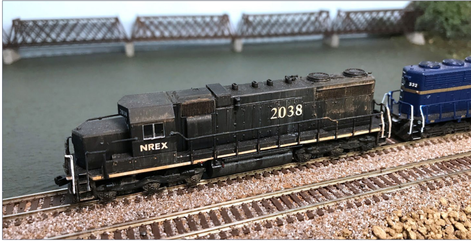
13. Conductor-side view of the finished unit, showing the unique placement of the bell, the Paducah short hood, and the liberated exhaust.
