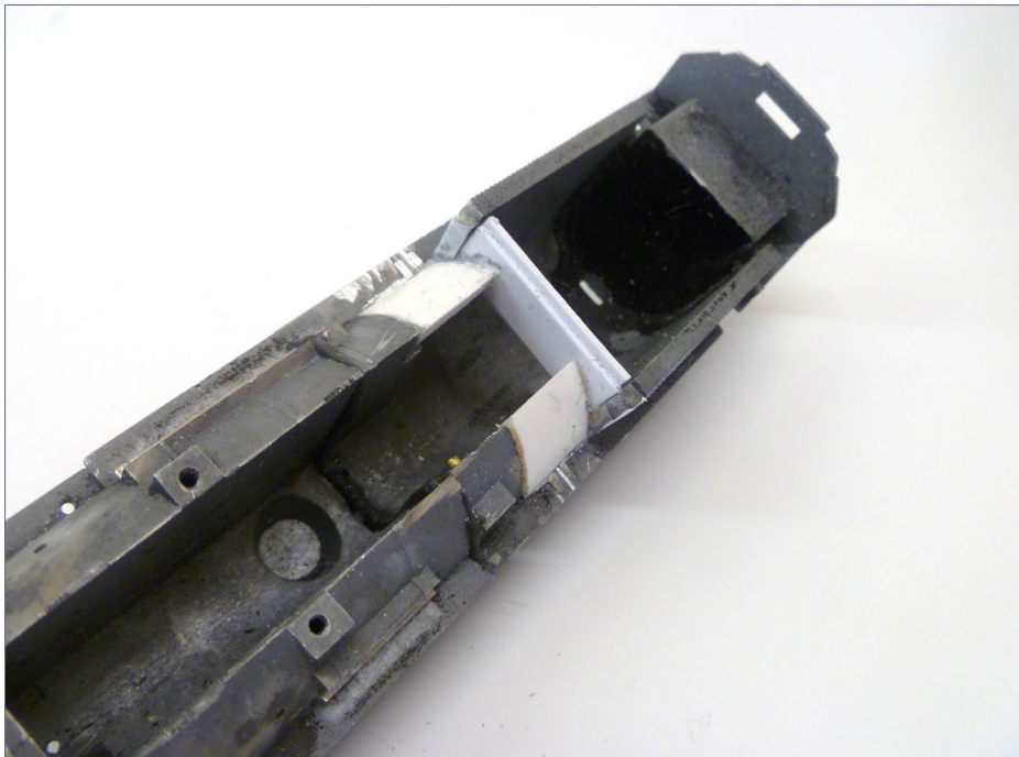
19. I installed styrene sheet to recreate the front of firebox. The center section will be cut away to clear the drive train.
