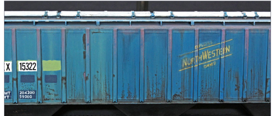
61. The car side appears quite grimy after several specifically applied, small area detail washes.
