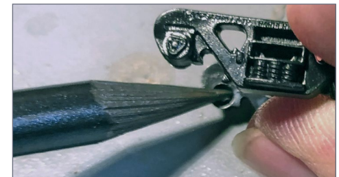
2. Burnish the axle tip holes with the 4B pencil.
