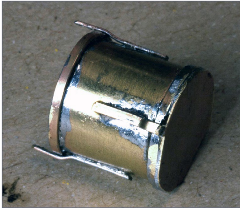
15. A completed coal bucket showing bottom, latch, and (barely visible) end of latch bar.
