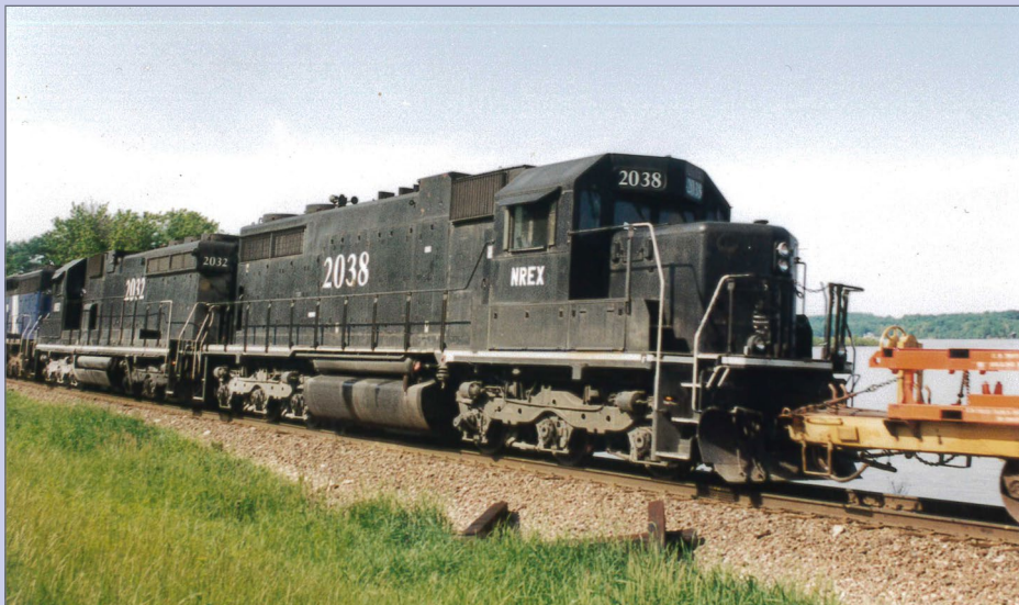
5. NREX 2038 at Princeton, Iowa, on the IMRL, May 22, 1999. This is one of four units rebuilt from SD35s, and the basis for my N scale model.
