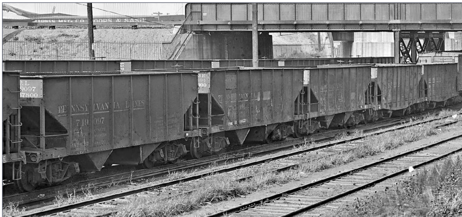
17. This 1921 photo of a string of Pennsy hoppers offers a rare view of the early 1920s lettering schemes and weathering. The first three are GLA cars and the last two are GL class. Check out the PENNSYLVANIA LINES lettering on the first car. The second car has had LINES painted out. Photograph by William B. Berry, Jr., from the Railfan.net Erie Lackawanna Email List Photo Archive
