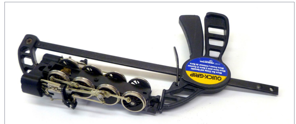
21. Epoxy and a bar clamp hold the pieces in place on rear frame.
