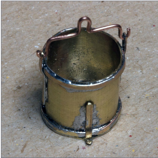
10. Here's my completed brass coal bucket with latch bar and latch at the bottom.
