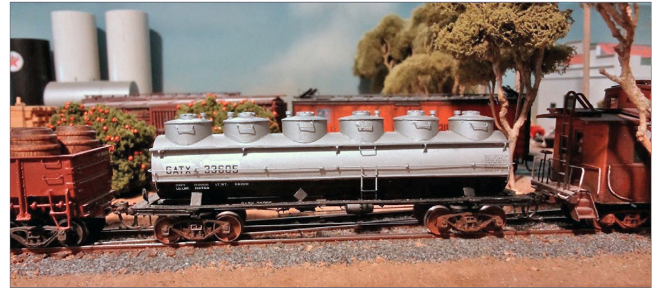
15. I scratchbuilt this version of a six dome tank with jacketed domes. The tank body is a piece of 3/4" copper pipe wrapped with 0.010" styrene sheet. The domes were made from an aluminum cigar tube. On my list of projects is a four-dome version.
