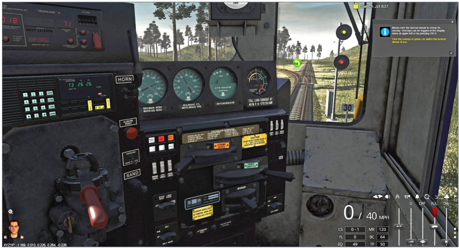
22. This shot was taken from inside the lead locomotive of the Rocky Mountaineer during the second tutorial. The selected train control mode lets the engineer operate the reverser, throttle, dynamic brakes, train brakes, and independent brake.
