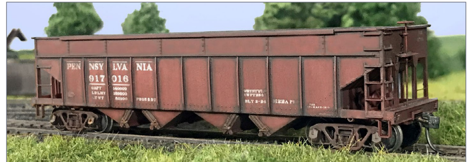
35. This is an older Bowser model of a H22a. The prototypes were originally built as a coke car. The Pennsy converted many for hauling coal. In addition to covering the original slatted coke gates, the car has been updated with 70-ton Crown trucks. I remember seeing these cars among H21a hoppers in the Pennsy's Sandusky, Ohio yard in the 1950s.
