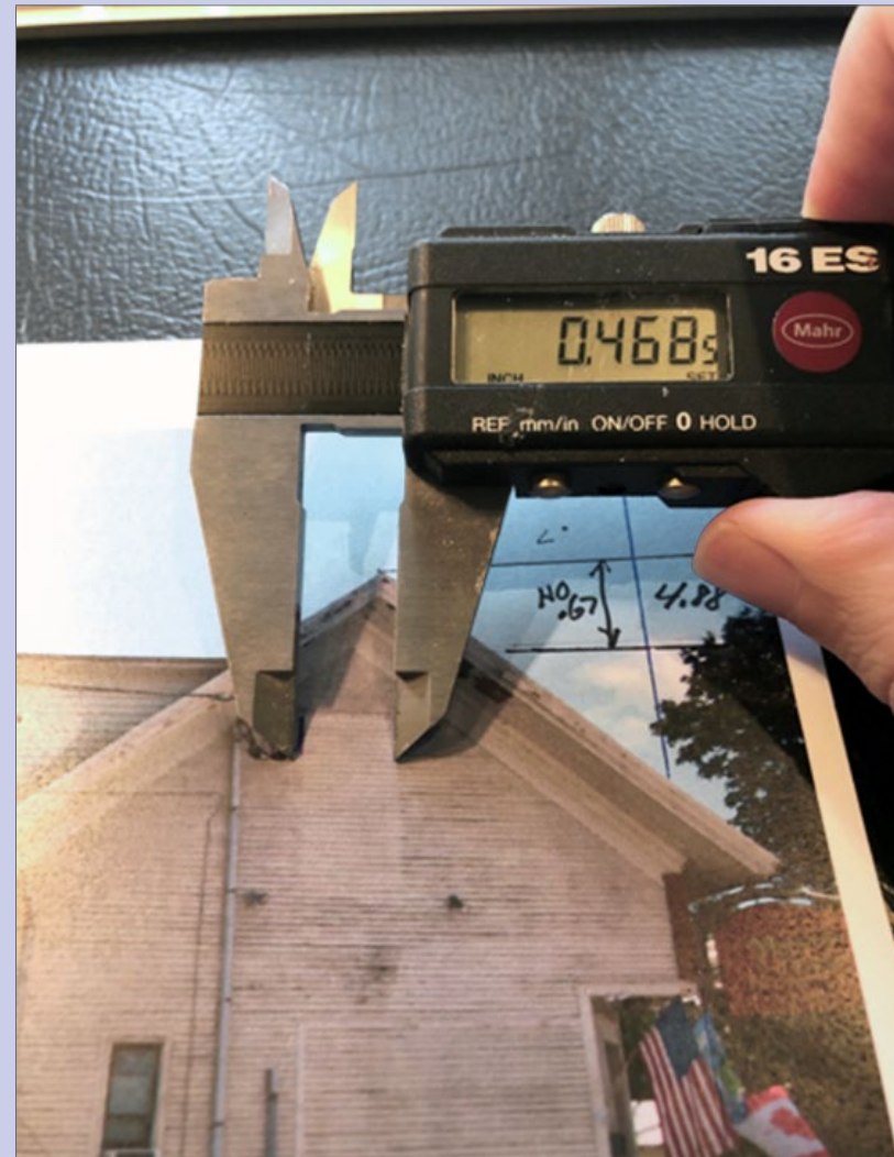
13. Specific modeling dimensions can be pulled from photos once a scale factor has been calculated.
