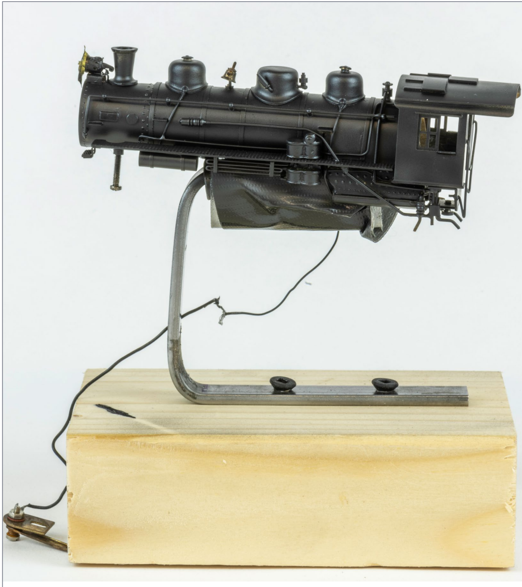
6. The boiler assembly after I sprayed a primer coat. The paint stands allow access to the model from all angles without holding it by hand. ☑
