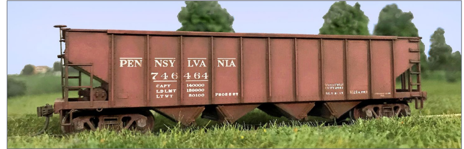
34. This pastoral scene catches PRR 746464 as it waits to be picked up for a trip back to the coal mines. A reinforcement angle was probably installed when the car was converted from clamshell to sawtooth hoppers. This lettering scheme was applied starting on May 14, 1926 and was standard until January 1930 when the circle keystone was added. The model is factory-painted by Bowser, but I removed the circle keystone. This car is not heavily weathered or beat up. It was recently shipped and repainted within the past year for my 1927 focus.
