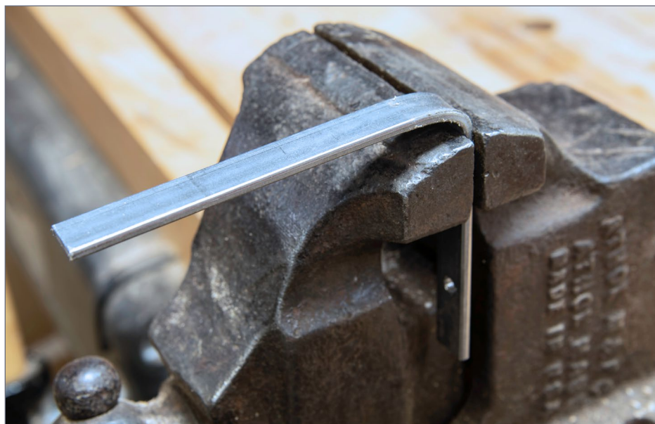
4. Using hand pressure, I made the first bend in the bar stock. The second bend was made in the same manner.
