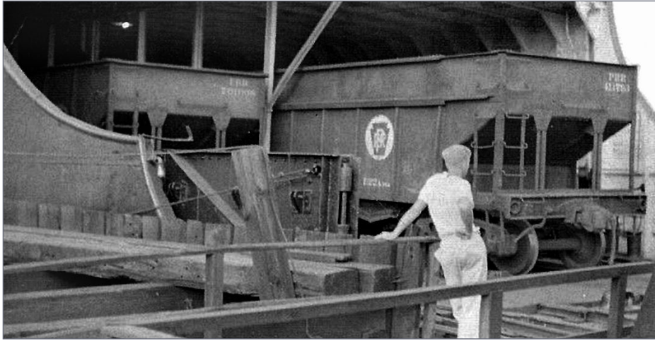
27. This late 1930s photo shows an H22a hopper. Note that there are two reinforcement angles. One is along the top of the car side, and another is just above the side stakes. The top reinforcement angle is heftier than the lower one. R. Biddy photo
