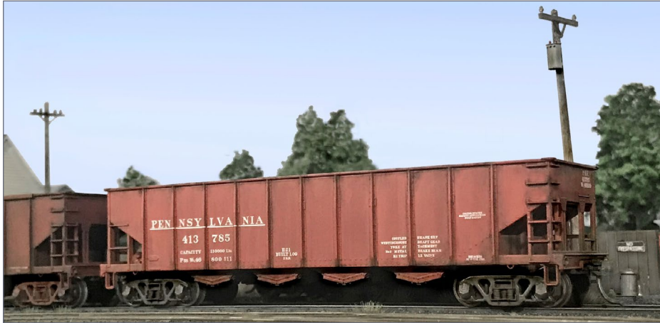
32. Another view of 413785 offers a better view of the Kadee No. 53 scale short-shank couplers. I weathered the model, but not as heavily as some of my other coal cars.
