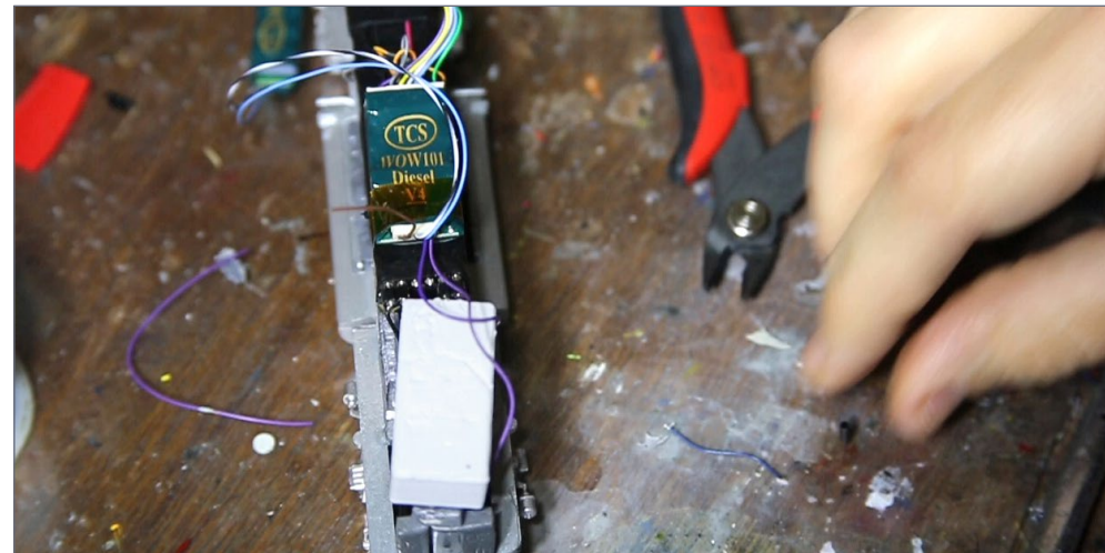
31. One purple wire from the decoder is routed to each end of the white speaker assembly. The speaker assembly is mounted to fire down through the rear truck well.
