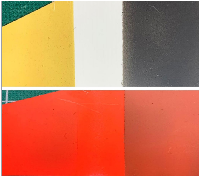
26. The top image shows Neutral Yellow Primer and white with Gray Stynylrez Primer. The bottom is Vallejo Red air-brushed over the above primer. Notice the color change over the gray primer.
