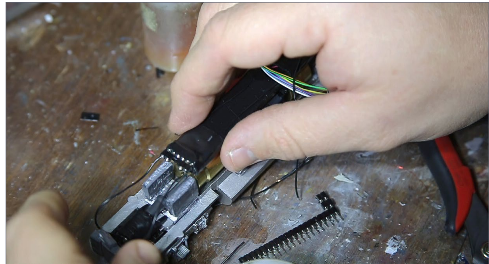
27. The decoder and weight are secured with double-side tape above the motor.
