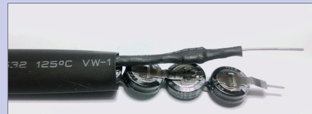
23. Shrink tubing installation.
