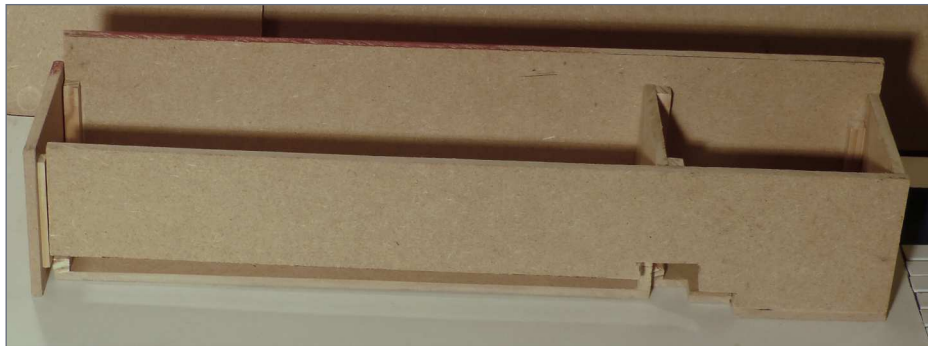
18. The shutter block housing assembled. Note the slot to allow the shutter movement.
