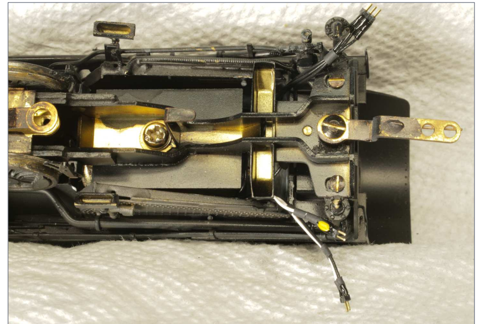
23. The chassis is assembled to the boiler with motor and light connecting wires seen under the cab.
