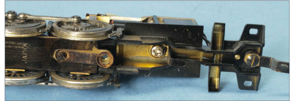
4. The screw holding the motor in place can be seen from the underside of the frame.
