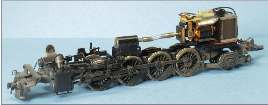
2. The original chassis with boiler and lead truck removed.
