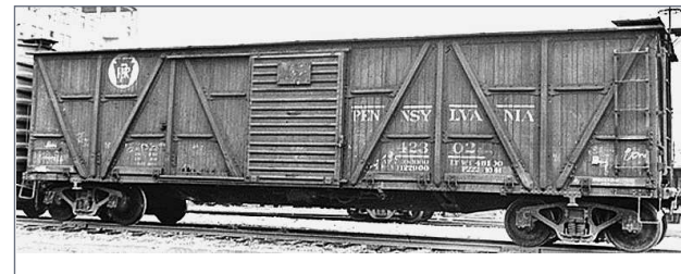
3. PRR 42302 X23 boxcar has been upgraded with a Youngstown corrugated metal door. The vertical wood sheathing is
