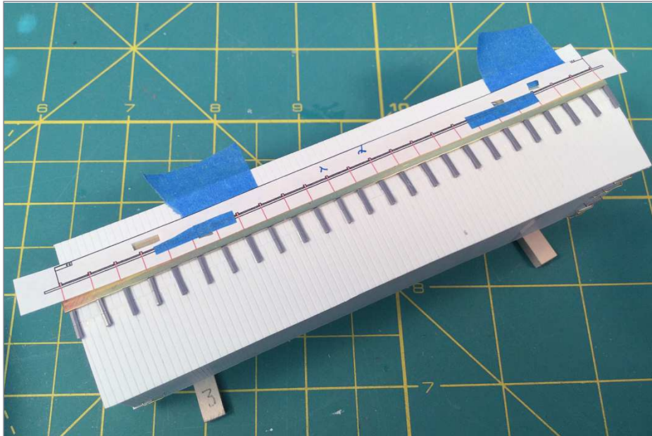
16. Completed roof supports on one of the six boxcars.
