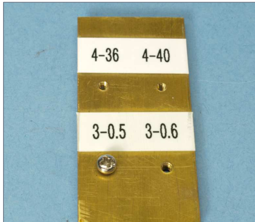
9. Here's my homemade tool to determine the size of the motor mounting screw.
