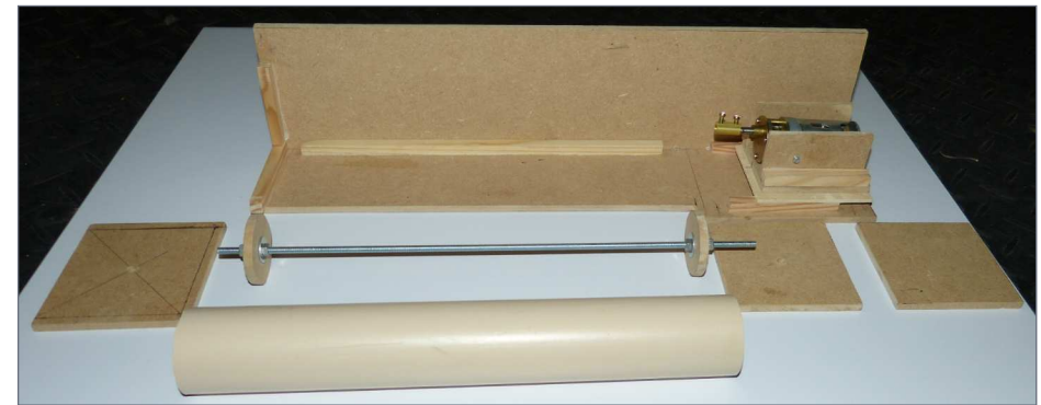
8. All the components of the shutter driving system.
