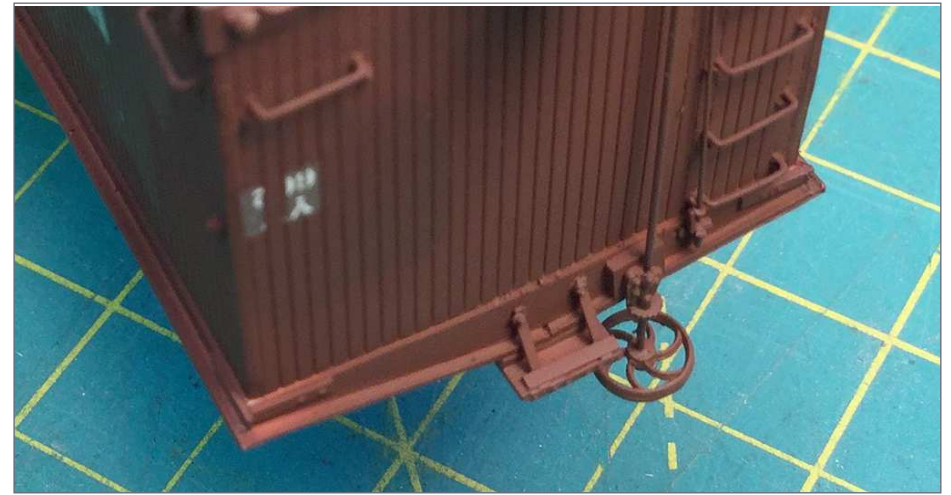
17. A close look at a photo-etched running board brace extending from the underside of the running board to the end fascia.
