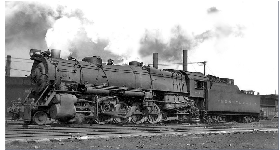
15. PRR 7036 at Delray, Michigan in 1948, is typical of the post-WWII N2sa class of locomotives. The original USRA tender has coal bunker extensions, as was typical for N2sa locos. The broader script in the tender indicates that it must have been re-lettered sometime after 1946. Ray Breyer collection
