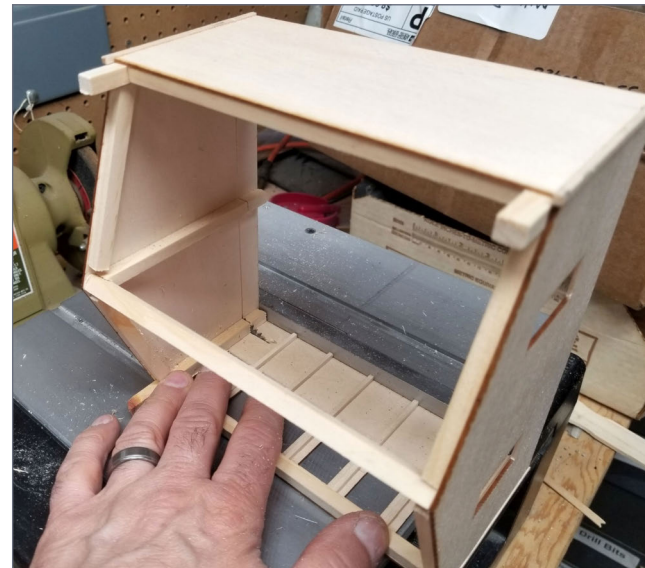
12. To shorten the clapboard structure, I set the fence of my Micro-Mark table saw to the width I wanted to remove and ran the completed building through the saw for all four sides. This was a quick, easy, and accurate way to shorten the building height.
