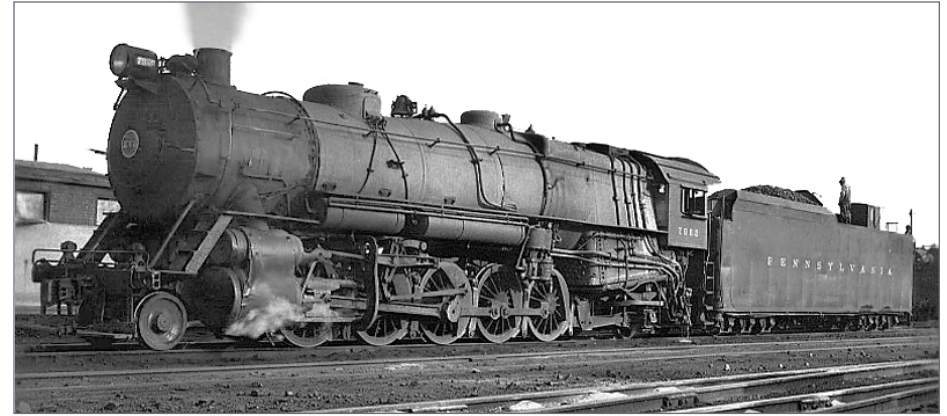
14. Pennsy 7962 sports a Pennsy "long haul" tender in place of its USRA tender in this 1946 photo from Chicago in 1946. This was not common of the N2sa locomotives. Ray Breyer collection
