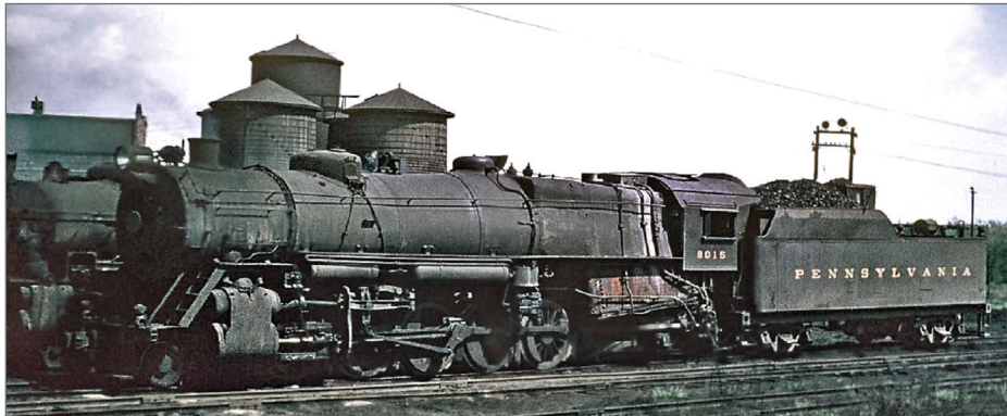
17. This rare color photo shows PRR N2sa 8015 at about 1950, near the end of its service life. This N2sa is looking tired, dirty, and rusty, but ready to work with a full load of coal in the tender.
