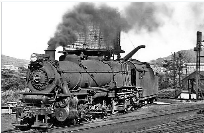
13. This photo was taken in West Reading, PA. The locomotive has been turned on the turntable and is taking on water and coal. This L1s is in its pre-1946 configuration. Ray Breyer collection
