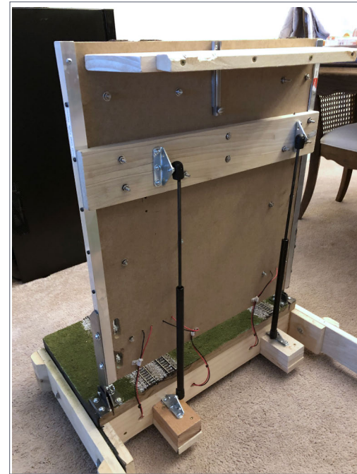
5. We used pneumatic struts to hold the gate open.
