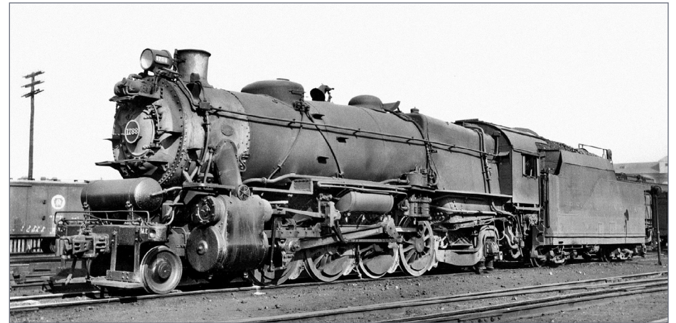
12. This is a good image of PRR 1788. There is a Train Phone antenna on the tender. The headlight and generator at the top front are in the post-WWII configuration that first appeared in 1946. Not all L1s locomotives got this treatment, but the majority did. Ray Breyer collection
