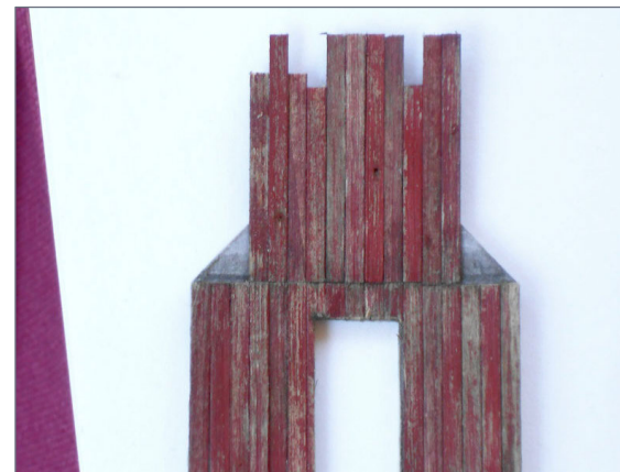
9. I applied the boards in the eaves end area, starting in the middle and working out.
