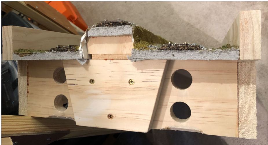
2. Wedge-shaped block on liftout. Note the access holes. They accommodate Allen wrenches to screws that adjust the receiving wedge's position.
