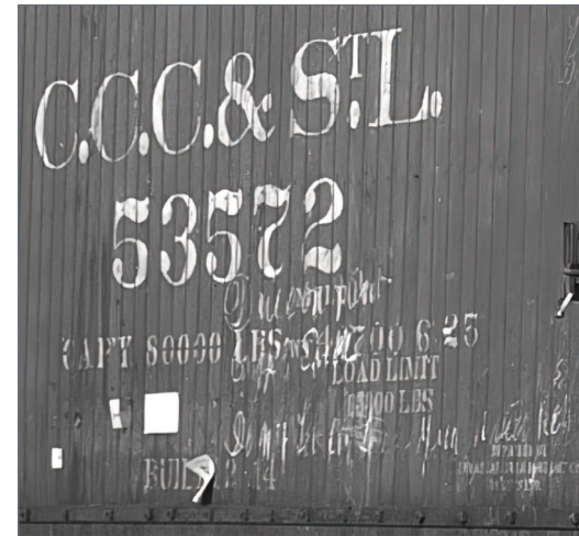
10. Another enhancement of [8] reveals an 80,000-pound load capacity.
