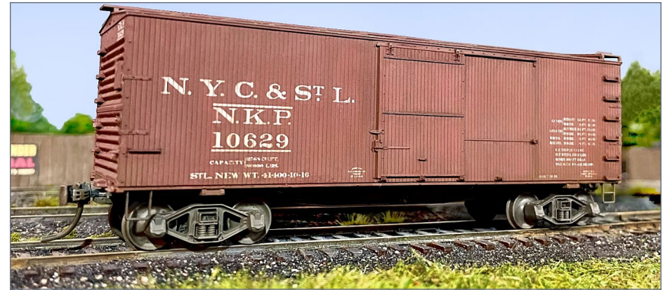
17. Accurail 1300-series model model. Factory paint, Kadee metal wheels, Kadee #153 scale couplers. Weathering with chalks wetted with decal setting solution.
