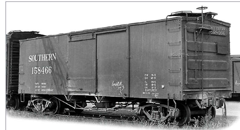
4. Southern 36-foot boxcar with stamped steel ends.
