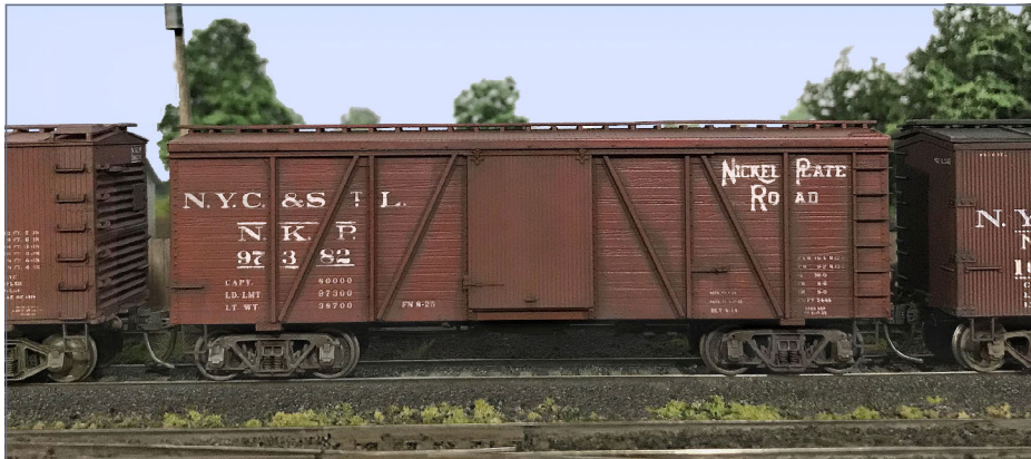
16. Accurail 1150-series model model. Factory paint, Kadee metal wheels, Kadee #153 scale couplers. Weathering with chalks wetted with decal setting solution.
