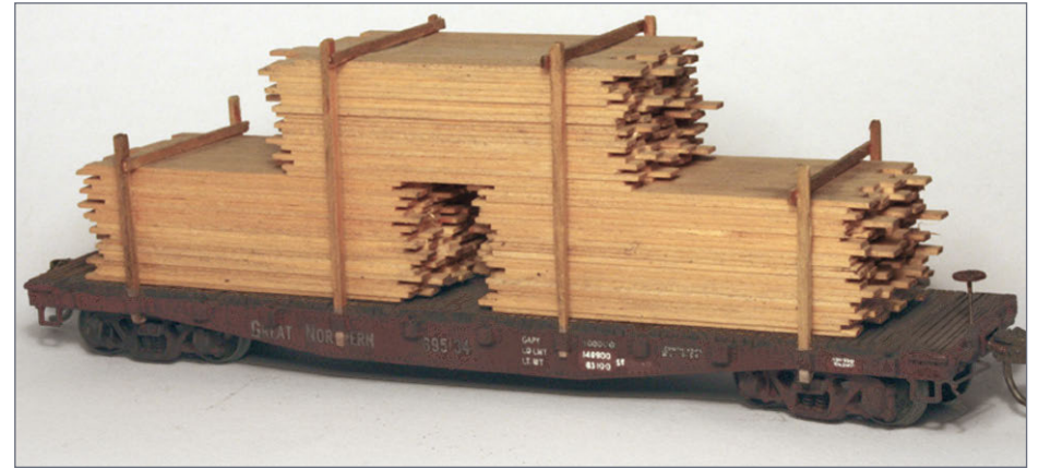
18. Lumber loaded this way, shown on a model of a Great Northern flat car, was usually rough. Any lumber yard without its own siding would receive this cargo at a team track.
