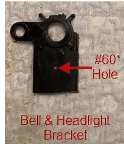
18. The bell and headlight bracket with a #60 hole for the wiring.
