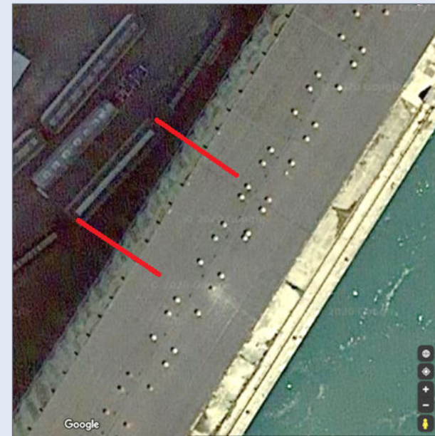
14. Hopper cars hidden in the shadows alongside the mill. The author used this reference, combined with the dimensions of a similar hopper car photographed at the mill [2], to scale the width of the silos.
