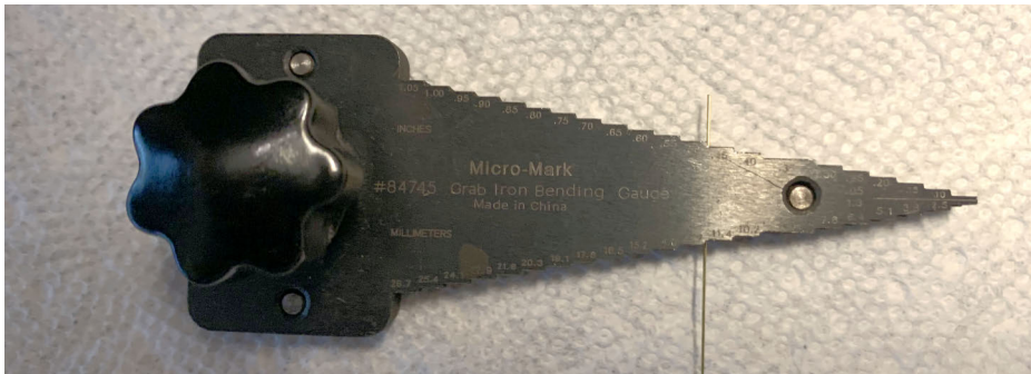
9. Bending wire to shape for cab handrails in Micro-Mark Grab Iron Bending Gauge.
