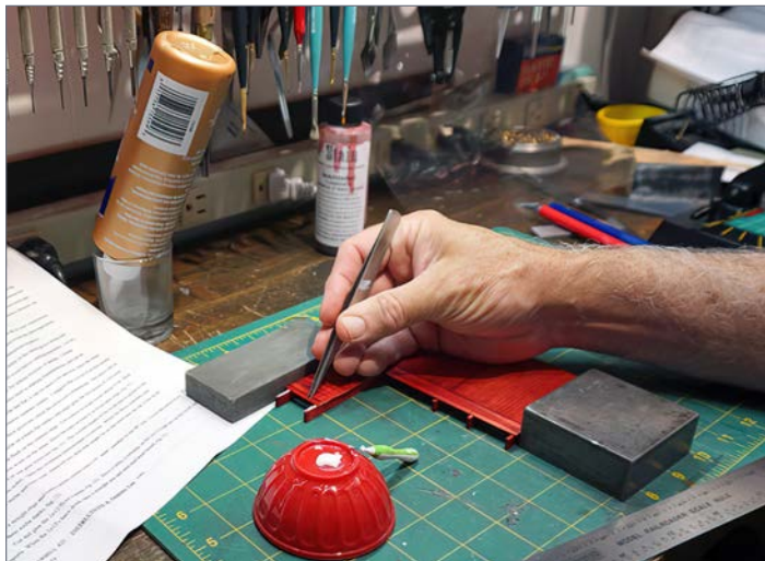
8. Gluing the floorboards to the joists.
