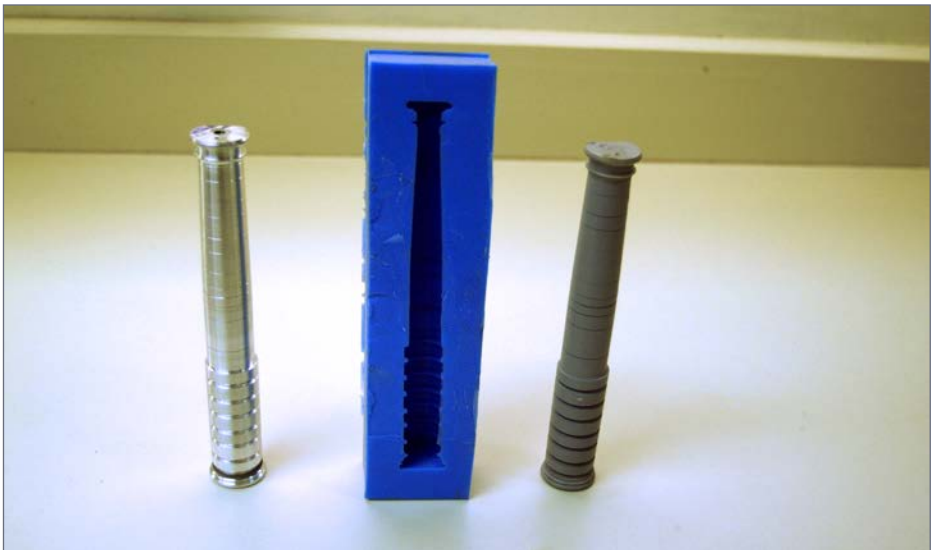
27. From left: the front column master, the mold, and first of six castings.
