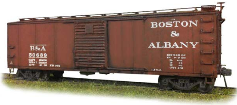
12. I weathered and re-lettered this BLI model of a Boston and Albany 40' steel boxcar from Standard Steel Car Company.
