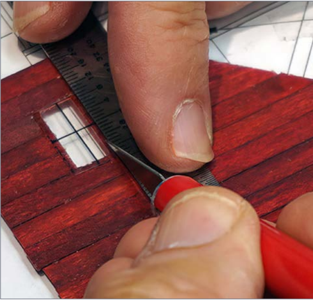
26. Trimming the windows.
